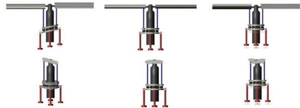
Figure 5: Swash-plate mechanism neutral position (center), collective input (right) and cyclic input (left)
