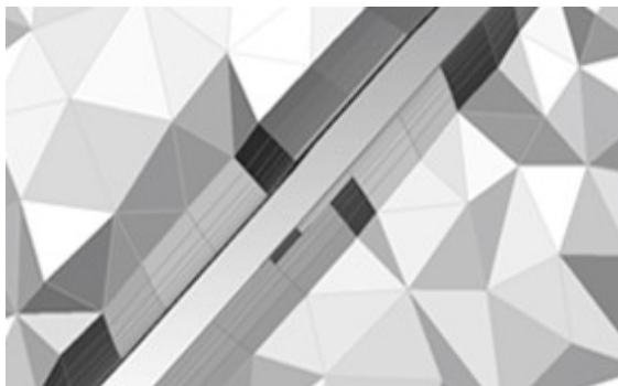
Figure 20. Prism mesh near the wall
