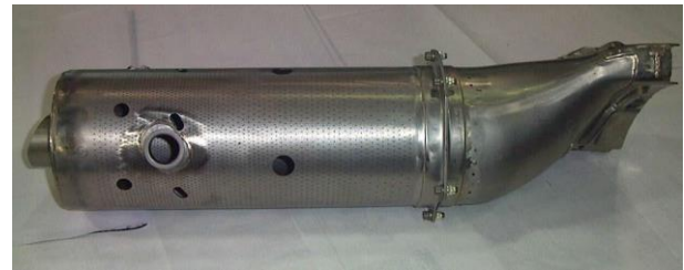
Figure 4. A picture of the 3.5 series combustion chamber
