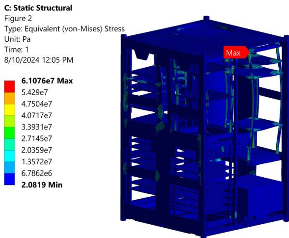
Fig. 11. Von Mises stress induced by quasi-static load.
