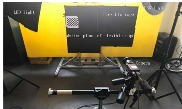
Figure 13. The experiment with the equipment for flexible rope visual measurement.
