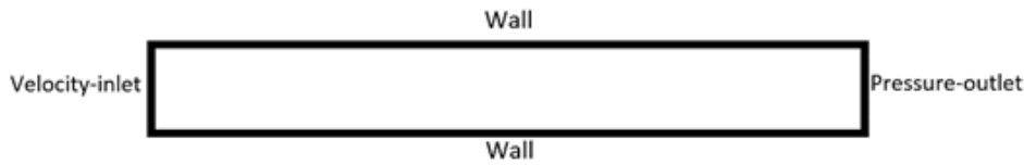
Fig. 4: Boundary conditions of Fluent model
