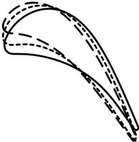
**Figure 5.** Rotor Blade Profile at Three Different Radii.
