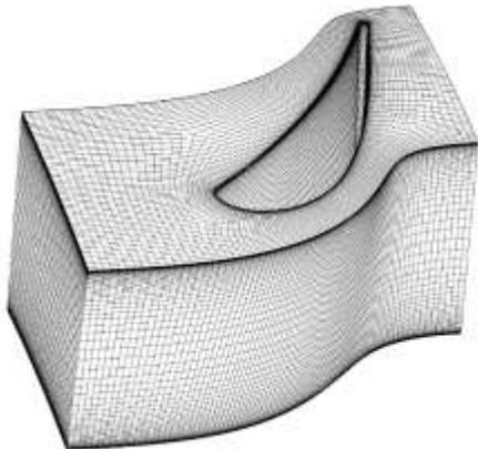
**Figure 6.** Computational Mesh for the Rotor.
