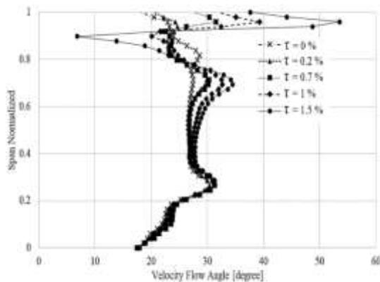
Figure 18. The radial distribution of the flow angle at the rotor exit.
