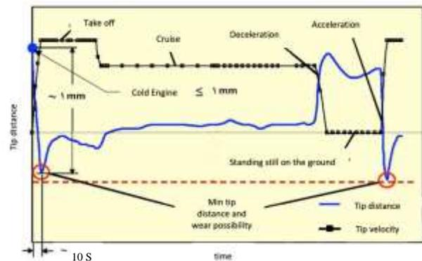
**Figure 2.** Changes in the distance between the blade tip during a typical flight [5].
