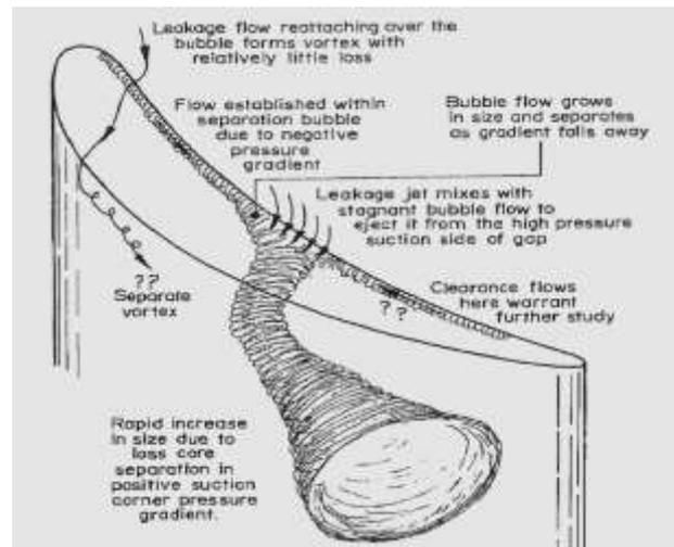
Figure 3. Conceptual model of the flow structure at the blade tip [10].
