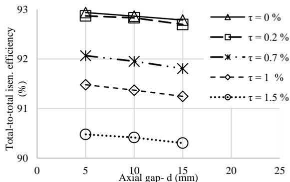
**Figure 22.** The variations in turbine efficiency with changes in the axial gap between the rotor and stator.
