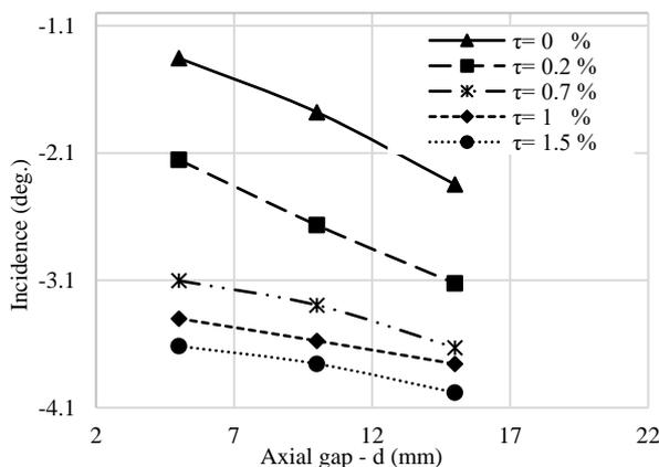
**Figure 21.** The changes in the angle of flow incidence on the rotor with changes in the axial gap between the rotor and stator.
