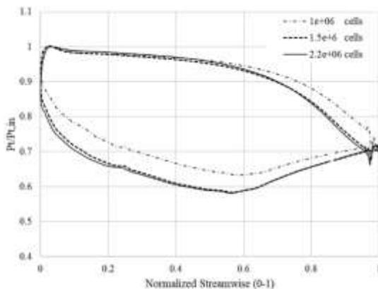
Figure 9. Pressure Distribution around the Blade to Investigate Mesh Independence.
