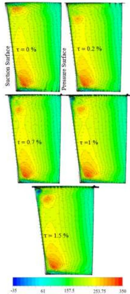
**Figure 17.** The relative velocity vectors along with axial velocity contours (m/s). One important aspect of turbine design is the angle of flow at the rotor exit, which is defined as follows:
