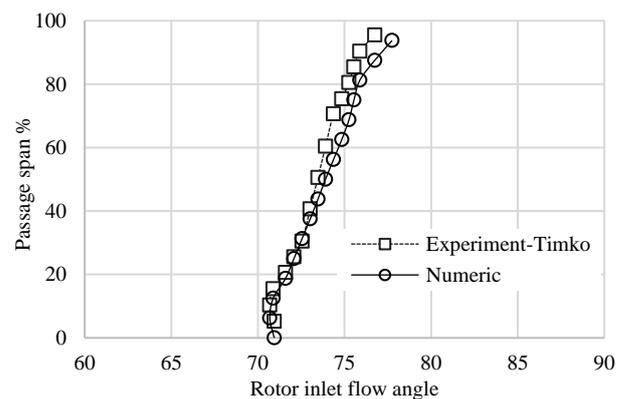
Figure 10. Flow Angle at the Inlet to the Rotor.
