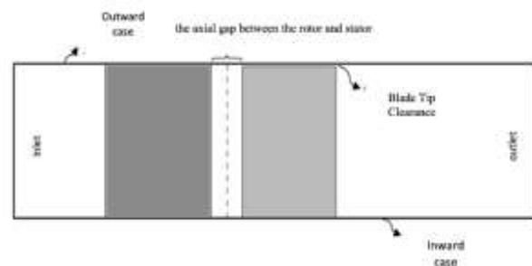
**Figure 4. 2D View of Flow Channel.**
