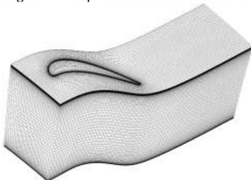
**Figure 7.** Computational Mesh for the Stator.
