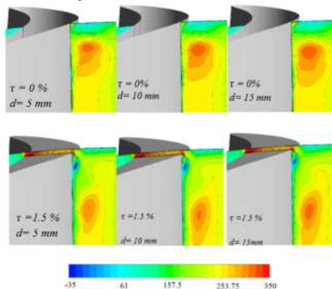
Figure 20. The axial velocity contours at the midpoint of the blade (m/s).
