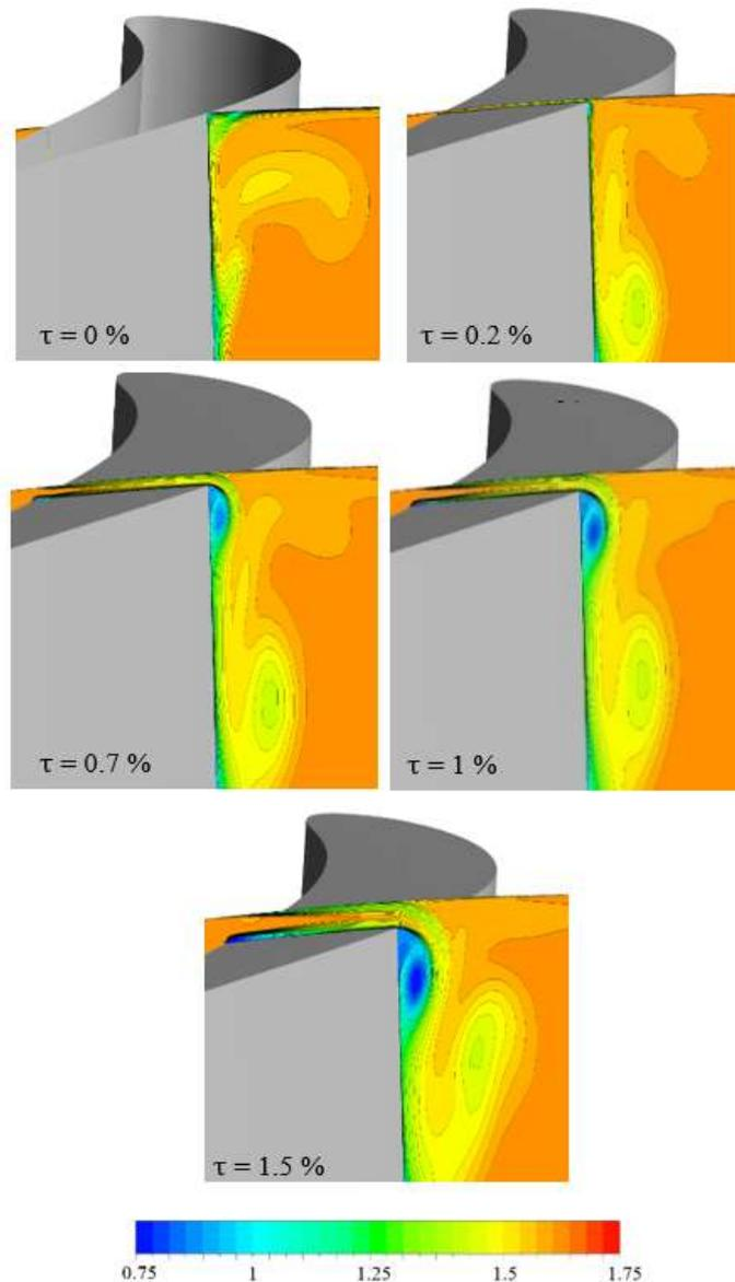
**Figure 15.** The total pressure contour ( $P_t/P_{amb}$ ) for different tip clearances in the middle of the blade.
