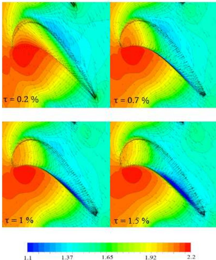
**Figure 13.** The static pressure contours (Ps/Pamb) along with relative velocity vectors.
