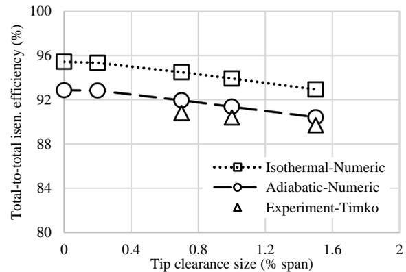
Figure 19. The variation in turbine efficiency with changing tip clearance of the rotor.
