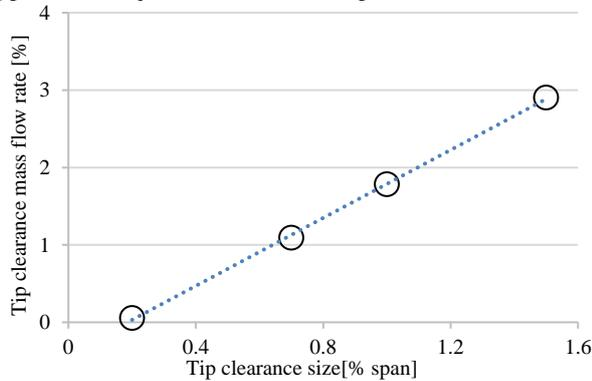
**Figure 12.** Leakage Mass Flow Rate (Normalized with Incoming Mass Flow Rate).
