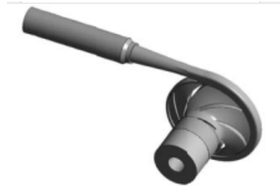
Figure 2 – computational domain for flow calculation passing through the pump
