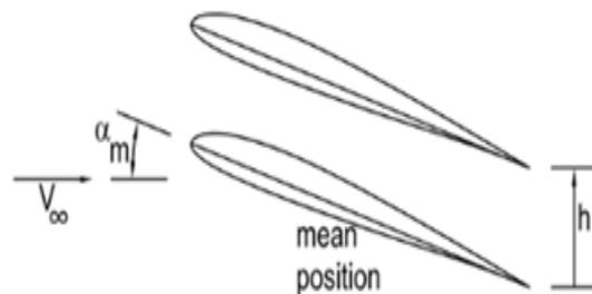
Figure 10. Pure plunge motion definition,  $\alpha_m=1^\circ$
