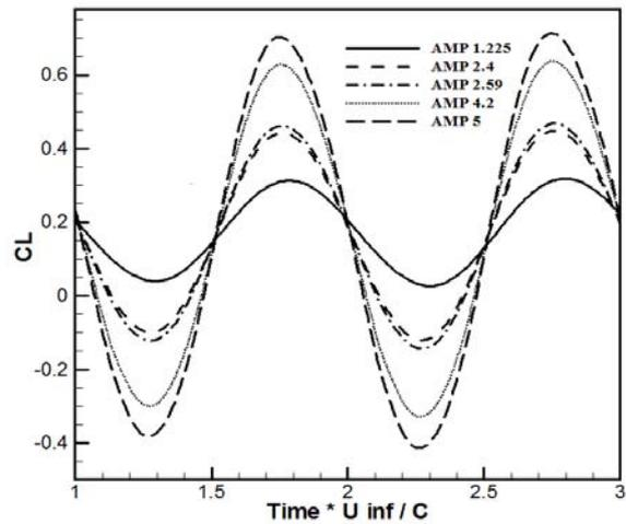
Figure 9. Instantaneous Lift coefficient versus non-dimensional time  $M_\infty=0.755$ ,  $k=0.0814$
