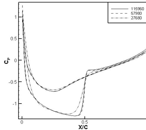
**Figure 5.** Grid dependency results for NACA0012,  $M_\infty=0.755$ ,  $\alpha=-1.8^\circ$
