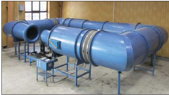
Figure 2. Schematic of the wind tunnel.
