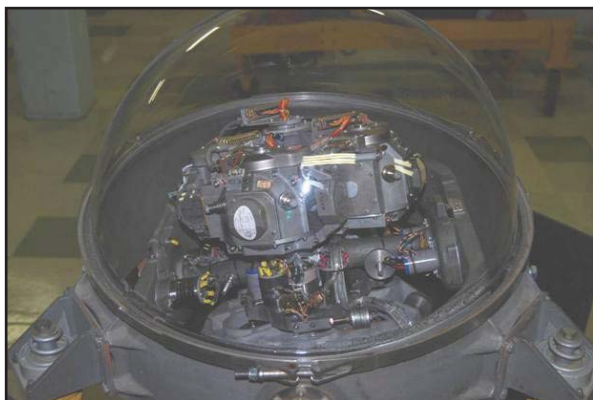
Figure 2. Real gimballed inertial measurement unit
