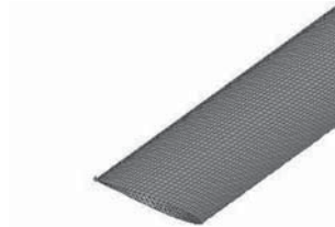
Figure 2. Surface Grids on Blade at \theta_c = +8 deg and MTIP = 0.877 .
