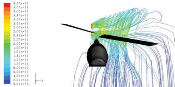
Figure 21. Tail Rotor Streamlines Colored by Velocity Magnitude – Dynamic Mesh.
