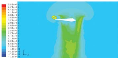
Figure 17. Pathlines Colored by Velocity Magnitude (m/s) Obtained by MRF.
