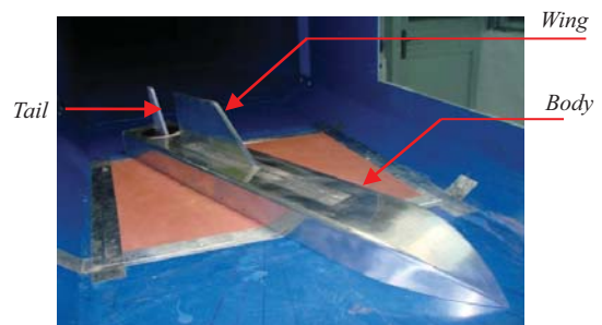
Figure 2. Model in the wind tunnel test section.
