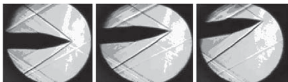
Figure 7. Schlieren images of the nose at M_\infty = 2.0 and various angles of attack.
