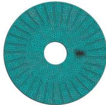
Fig. 5. A view of the meshing of the entire disc containing a radial crack with an aspect ratio of 0.4
