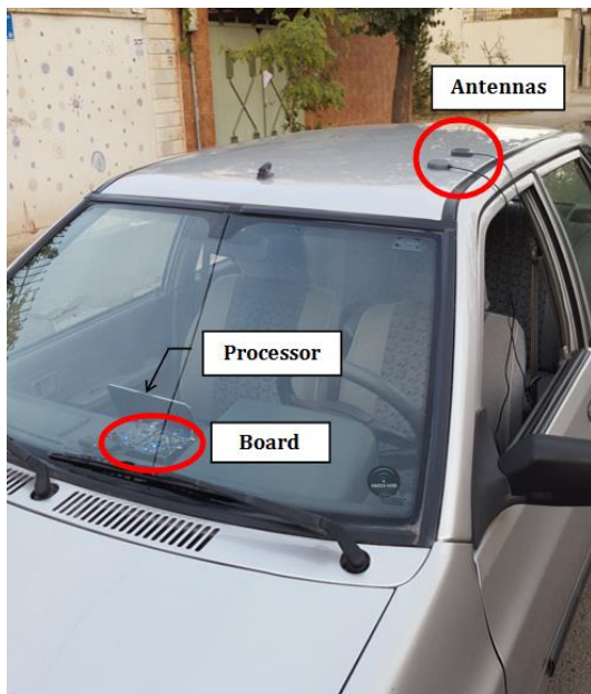
(Continuation) Figure 5. Mounting the hardware on the test vehicle.
