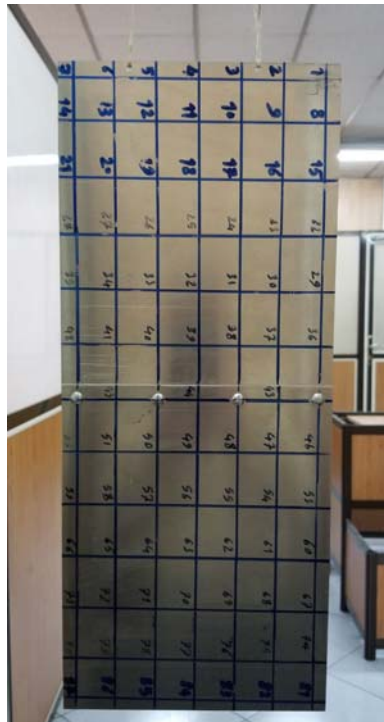
Fig. 2 Setup of experimental modal test conducted on the riveted lap joint 165x151mm (220 x 220 DPI)
