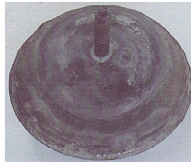
Figure 7. Other sample workpieces with different configurations shaped superplastically
