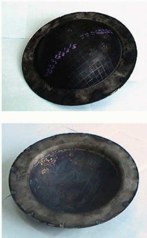
Figure 6. Lens-shaped workpieces shaped superplastically
