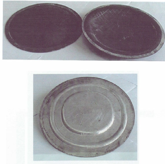
Figure 7. Other sample workpieces with different configurations shaped superplastically
